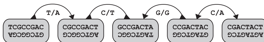
Figure 2.1 The four ways in which nodes are connected in the bidirected de Bruijn graph, with the edges labeled with the initial characters in the bidirected k -string graph (before edge compaction).
